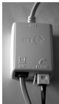
Figure 11.2: A typical ADSL microfilter
